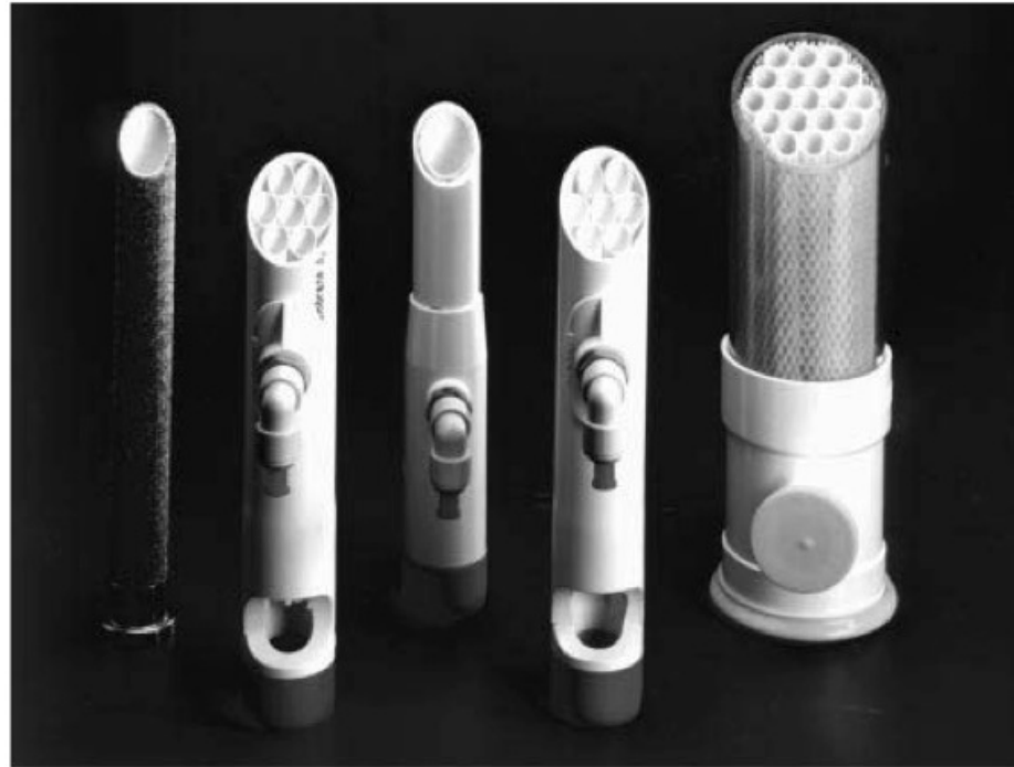
Figure 3.54 Typical tubular ultrafiltration module design. The membrane is usually cast on a porous fiberglass or paper support, which is then nested inside a plastic or steel support tube. In the past, each plastic housing contained a single 2–3 cm-diameter tube. More recently, several 0.5–1.0 cm-diameter tubes, nested inside single housings, have been introduced. (Courtesy of Koch Membrane Systems.)
