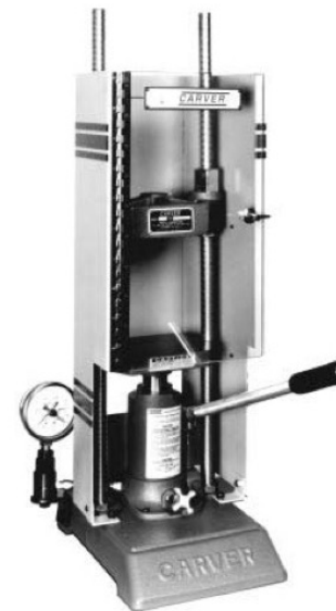
Figure 3.3 A typical laboratory press used to form melt-pressed membranes. (Courtesy of Carver, Inc., Wabash, IN.)
