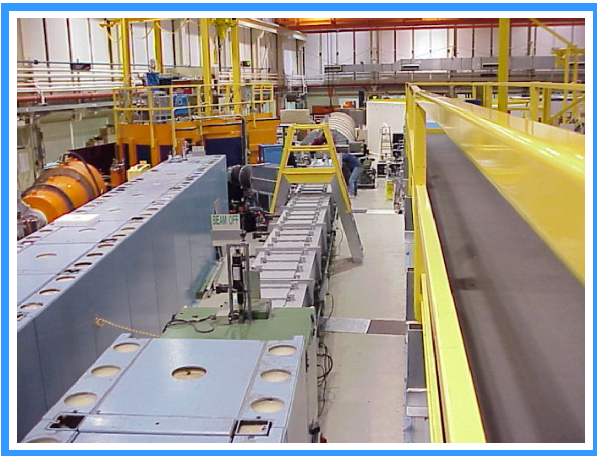
Figure 7: Photograph of the NG3 30 m SANS instrument. The picture was taken from the cat walk just before the velocity selector shield.
