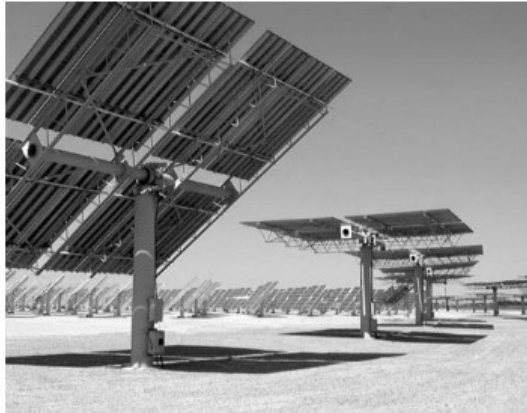
FIGURE 3.22 Detail of a heliostat.
