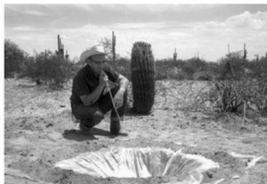
Figure 7-5 A solar still in operation. Image courtesy © U.S. Department of Agriculture—Agricultural Research Service.
