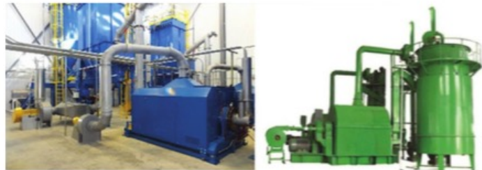
FIGURE 7.10 Ball mill. (From MAC Engineering. Available at http://www.mac-eng.com ; Leader Tech United. Available at http://www.ltucompany.com .)
