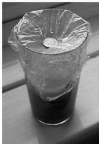
Figure 7-2 Demonstration solar still.
