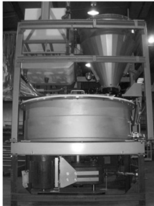
FIGURE 7.11 Vertical muller mixer. (From MAC Engineering. Available at http://www.mac-eng.com .)
