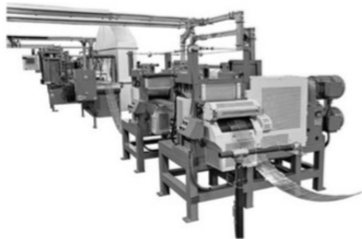
FIGURE 7.6 Continuous grid caster. (From Wirtz Manufacturing. Available at http://www.wirtzusa.com .)
