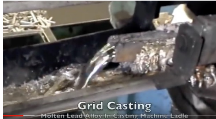
Molten Lead Alloy In Casting Machine Ladle
