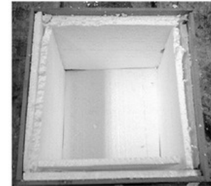
Figure 6-7 The box lined with polystyrene.
