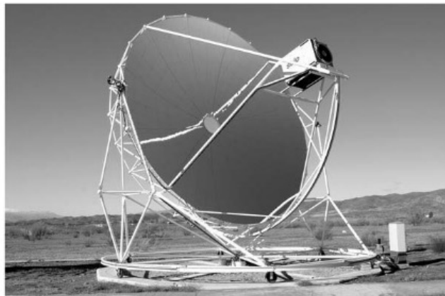
FIGURE 3.20 Parabolic dish collector. (a) Schematic diagram. (b) Photo of a Eurodish collector (from www.psa.es/webeng/instalaciones/discos.html ).
