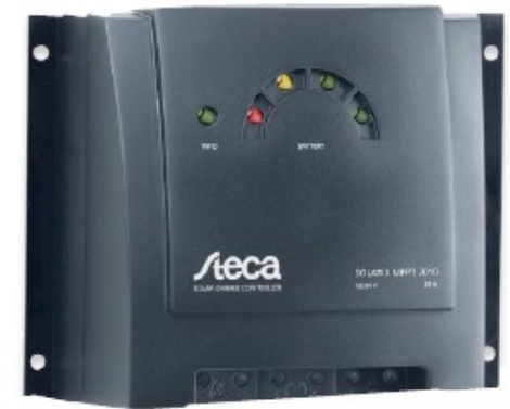
Figure 5.9 This MPPT controller can control a 12 or 24 V system with PV array power up to 500 W p and MPP voltages up to 100 V. With dimensions 19 × 15 × 7 cm, it weighs 900 g (Steca Elektronik GmbH).
