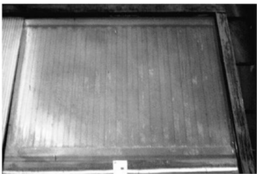
Figure 4-9 A recycled radiator collector.
